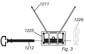
Step 2: Using the adjustment pin attach the tire stop to the front post
